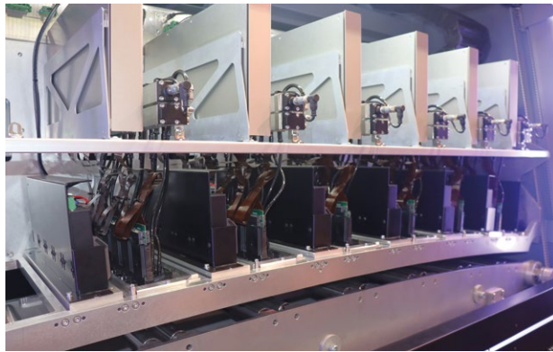
CMYK printhead array with orange and violet. (Source: pack.consult)
